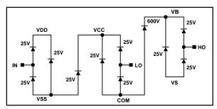
Figure 10. IR2110 Parasitic Diode Structure
