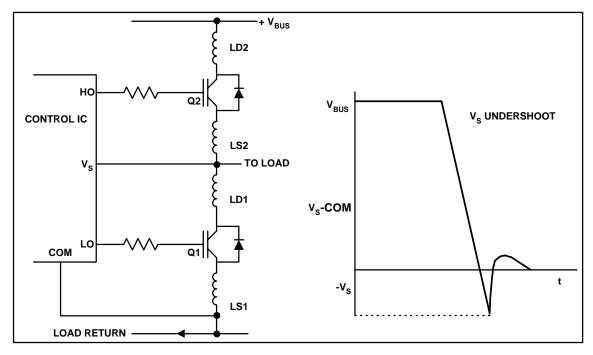
Figure 1. Parasitic Elements of the Half Bridge
