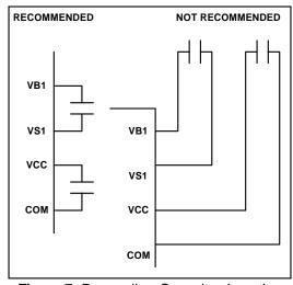
Figure 7. Decoupling Capacitor Location
